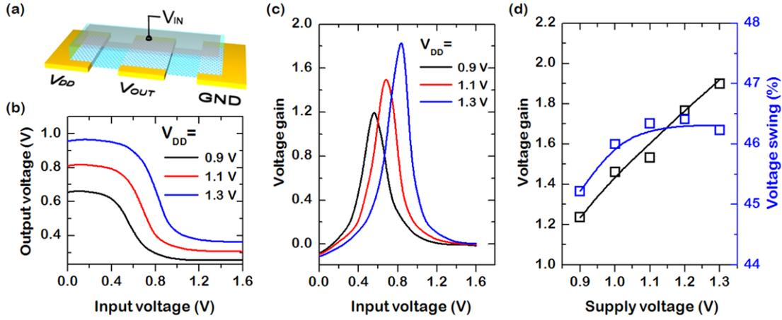
**Figure 3.** (a) Schematic diagram of a complementary inverter based on two graphene transistors with photo-patternable ion gel gate dielectrics. (b) Voltage transfer characteristics and (c) corresponding voltage gain of a complementary graphene inverter at three different values of  $V_{DD}$  (0.9, 1.1, and 1.3 V). (d) Voltage gain and swing of a complementary graphene inverter as a function of  $V_{DD}$ .
