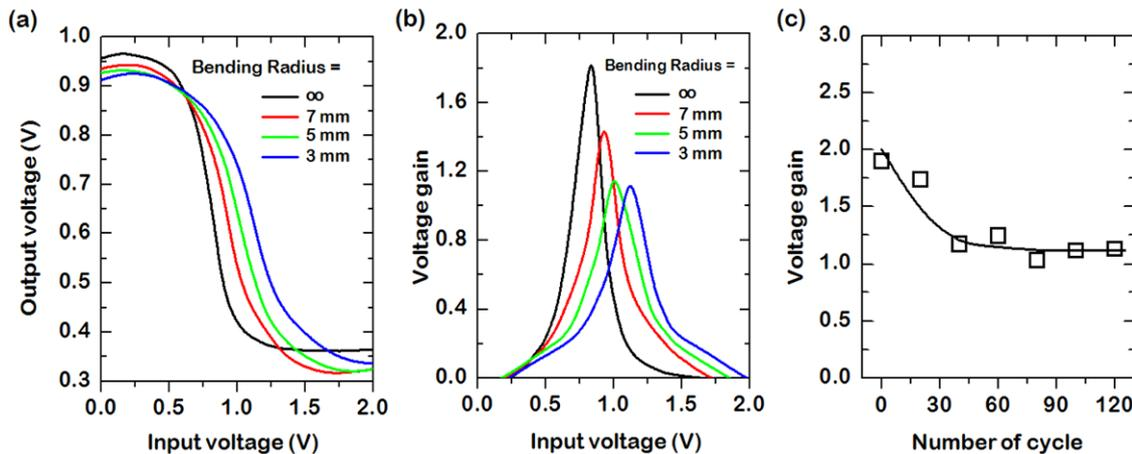
**Figure 4.** (a) Voltage transfer characteristics and (b) corresponding voltage gain of a complementary graphene inverter as a function of bending radius (7, 5, and 3 mm). (c) Voltage gain as a function of cycle (bending radius = 5 mm).
