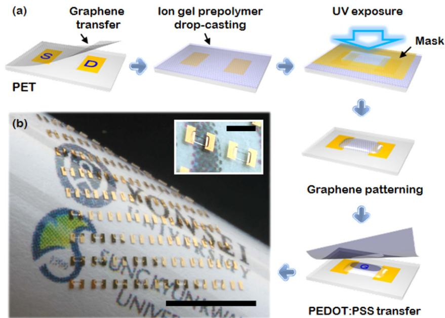
**Figure 1.** (a) Schematic diagram of the fabrication procedure for flexible graphene transistors with photo-patternable ion gel gate dielectrics on a PET substrate. (b) Large-area flexible graphene transistor array (scale bar: 5 mm). The inset shows the optical image of a completed device unit (scale bar: 1 mm).
