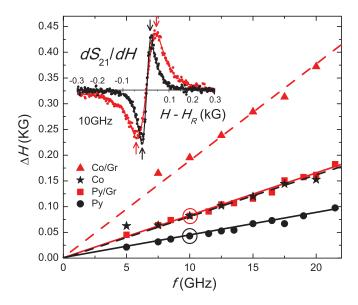
FIG. 3. Frequency dependence of the FRM linewidth for Py, Py/Gr, Co, and Co/Gr films obtained with the magnetic field applied at  $\theta = 0$  (in-plane configuration). The inset shows the field derivatives of CPW S<sub>21</sub> transmission parameter (at 10 GHz) of the Py and Py/Gr samples, from which the linewidth,  $\Delta H$ , is calculated as the peak-to-peak distance.
