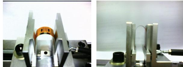
Fig. 4. Equipment for bending experiment.
