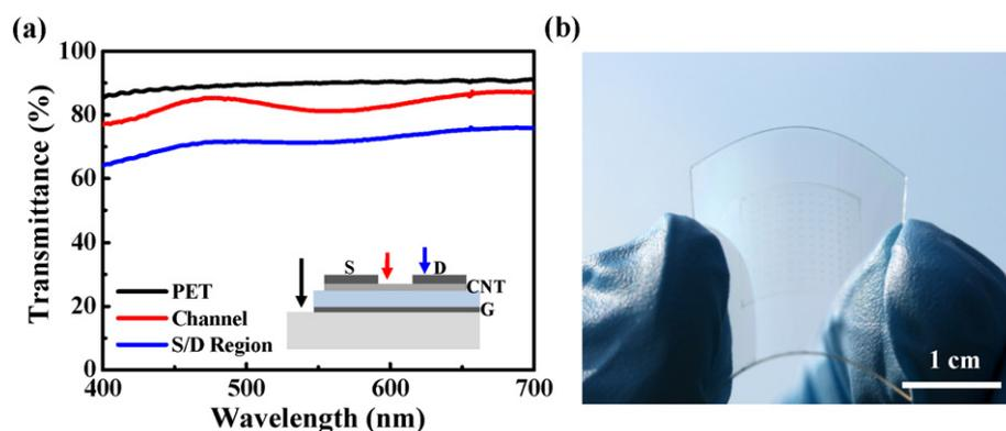
**Figure 2.** (a) Optical transmittance as a function of wavelength for the PET substrate (black line), through the channel region (red line) and through the source/drain electrode (blue line) of the device including PET substrates. (b) Optical images of a completed array of the TTFTs on the PET substrate.
