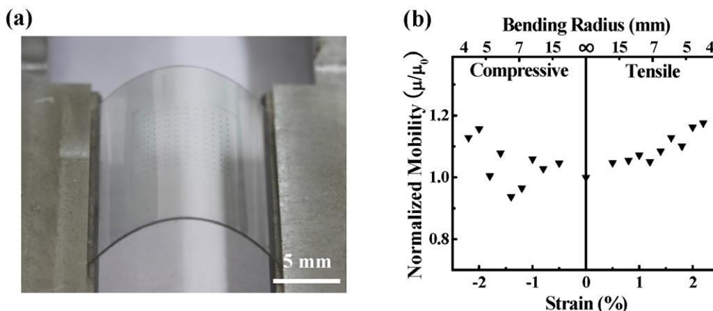
**Figure 4.** (a) Optical image during the bending test. (b) The change in the normalized effective device mobility  $\mu/\mu_0$  for TTFTs as a function of the bending induced strain and bending radius.
