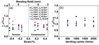
Fig. 3. (a) Normalized effective mobility  $(\mu_{\rm eff}/\mu_{0\,\rm eff})$  as a function of bending-induced strain and bending radius. (b) Normalized effective mobility after bending (to 3-mm radius; 0.44% strain) and unbending the devices several thousand times.
