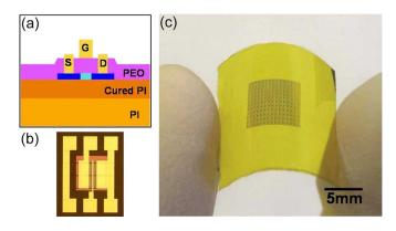
Fig. 1. (a) Schematic cross-sectional view of a single-crystal silicon TFT on PI (PI;  $25-\mu m$  thick) with a SiO<sub>2</sub> layer deposited by low-temperature PECVD as a gate dielectric (PEO; 100-nm thick). (b) Optical-micrograph top view of a typical device. (c) Optical images of an array of devices on a plastic substrate.
