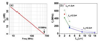
Fig. 4. (a) Experimental plots of  $H_{21}$  obtained from TFT of  $L_c = 2 \mu m$  and  $L_o = 1.5 \mu m$  with  $V_g = 2 V$  and  $V_d = 2 V$ . (b) Dependence of  $f_T$  on the gate length of TFTs: Measured (filled) and calculated values (open).
