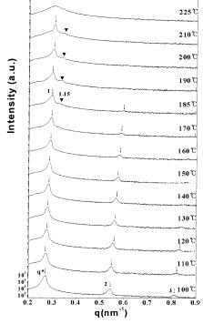
Figure 3. SAXS profiles of unsheared PSI67/PI7K blend as a function of temperature at the rate of 2 °C/min.
