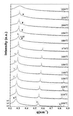
**Figure 2.** SAXS profiles of unsheared PSI67/PI3K blend as a function of temperature at the rate of 2 °C/min.
