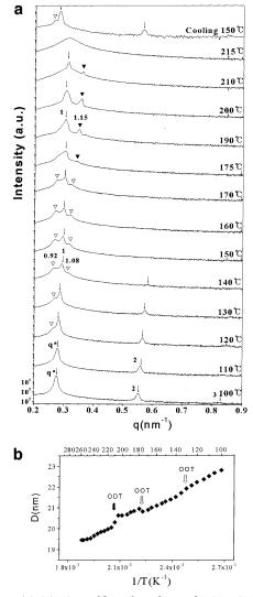
**Figure 1.** (a) SAXS profiles of unsheared PSI67/PI1K blend as a function of temperature at the rate of 2 °C/min. SAXS pattern observed during heating process was not much different from that after extended isothermal annealing. (b) Plot of interdomain distance  $D (=2\pi/q^*)$  vs 1/T. The  $T_{\text{ODT}}$  and  $T_{\text{OOT}}$  are indicated by filled and open arrows, respectively.
