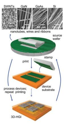
**Fig. 1.** Schematic illustration of a printed semiconductor nanomaterials—based approach to heterogeneous 3D electronics. The process involves the repetitive transfer printing of collections of nanotubes, nanowires, nanoribbons, or other active nanomaterials, separately formed on source substrates, to a common device substrate to generate interconnected electronics in ultrathin, multilayer stack geometries. HGI, heterogeneous integration.
